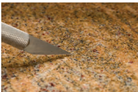
Hardened steel and quartz (granite) have the same hardness rating.
